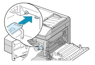
**5** Reinstall the toner cartridge, then lock the lever.
